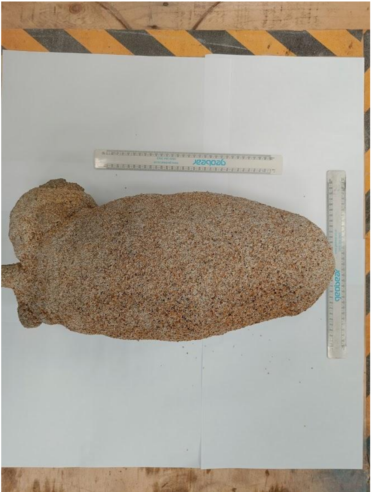
Figure 1. Geopolymer bulbs injected in granular soil
