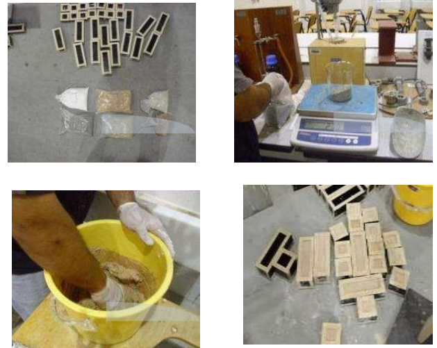
Figure 4: Steps to use to produce the new mortar
