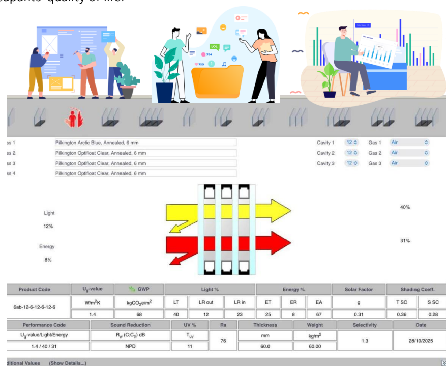
Figure 1 shows the online mobile app for quadruple glass (spectrum.pilkington.com, 2025)
