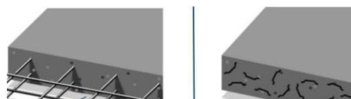
Figure 3 - Conventional vs Steel Fiber Slab
