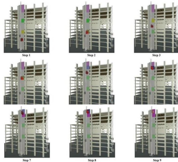
Figure 4. Temporary elevator operation planning simulation
