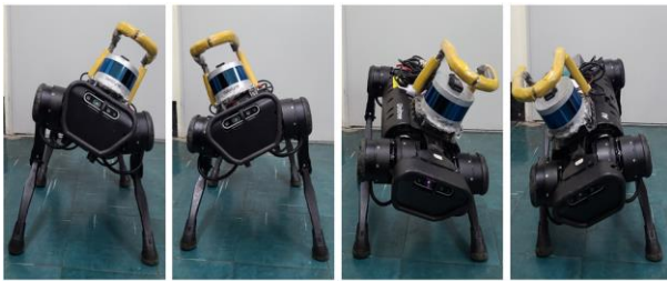
Figure 3. Examples of robot dog scanning postures
