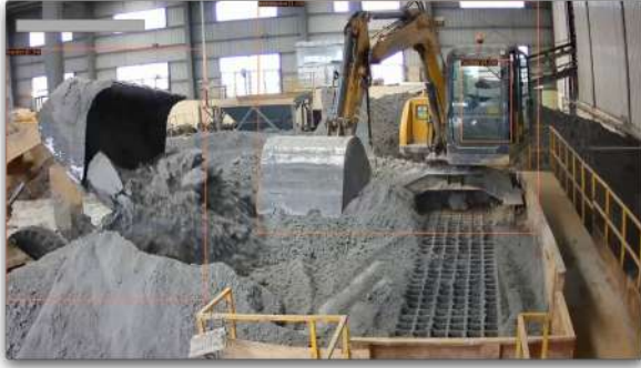
Figure 6. Detection result. Our system is capable detecting multi-class construction machines and human in real-time.
