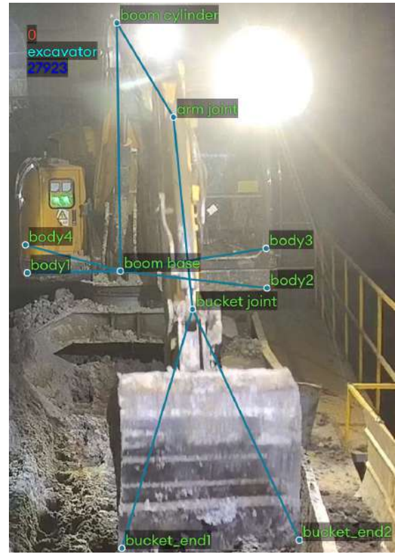
Figure 2. Excavator and corresponding pose labels. We labeled 10 parts of excavators including 2 bucket end keypoints (bucket end1, bucket end2), bucket joint, arm joint, boom cylinder, boom base and 4 body keypoints (body1, body2, body3, body4).
