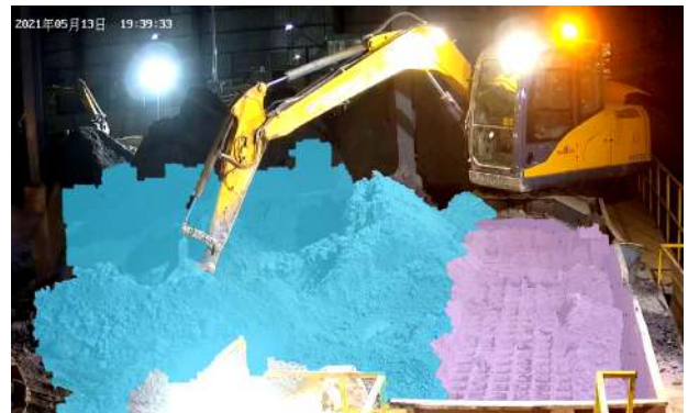
Figure 3. Area segmentation. The pink color area is dumping area and the blue color area is digging area.
