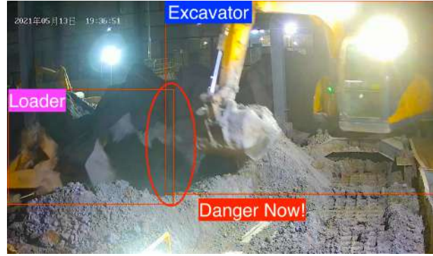
Figure 4. The autonomous excavator and loader potential collision scene when loader tries to load in digging area. The danger signal is sent when the autonomous excavator and the loader machines are both detected in the digging area.
