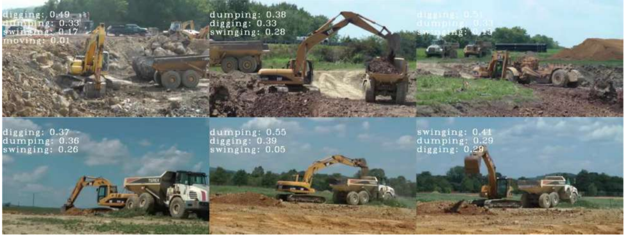
Figure 9. Long video demos of action recognition result on different scenes of the construction dataset. Prediction with the highest possibility is showing in the first line.
