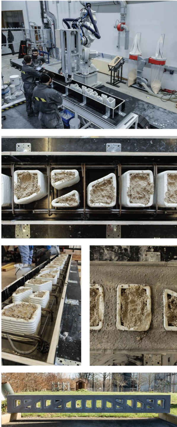
Figure 6. Fabrication of the second prototype. From top to bottom: printing of the moulds, insertion of the rebars and filling of the moulds with sand, pouring of the concrete, demoulded beam.
