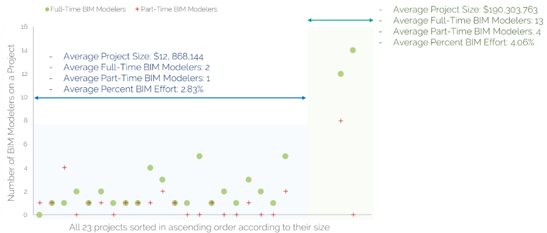
Figure 3. Overview of the allocation of electrical contractors' BIM resources on construction projects
